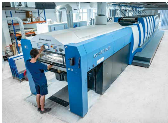
Printer Marco van Laak enjoys working on the fully automated eight-colour press with 4/4 perfecting and an additional coating unit
