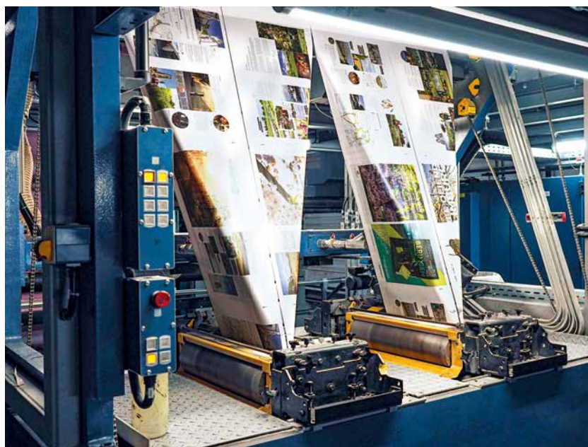
The adjustable formers of the Cortina allow CPP to offer a diversity of newspaper formats
