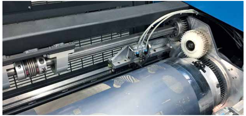
Rotary screen in the printing unit of the Rapida RSP 106
