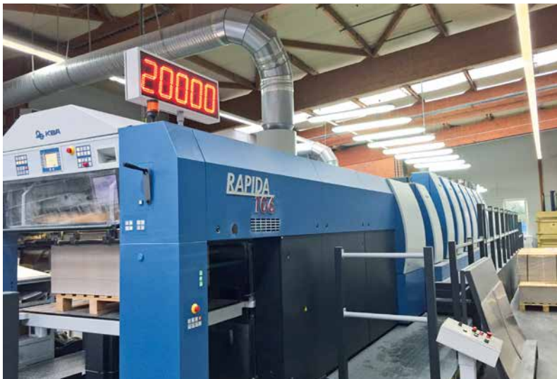
The new Rapida 106-7+L in the high-speed version reaches an incredible 20,000 sheets per hour
