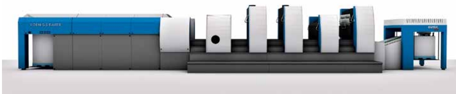
Printing and finishing with coater, intermediate drying towers and a screen printing unit
