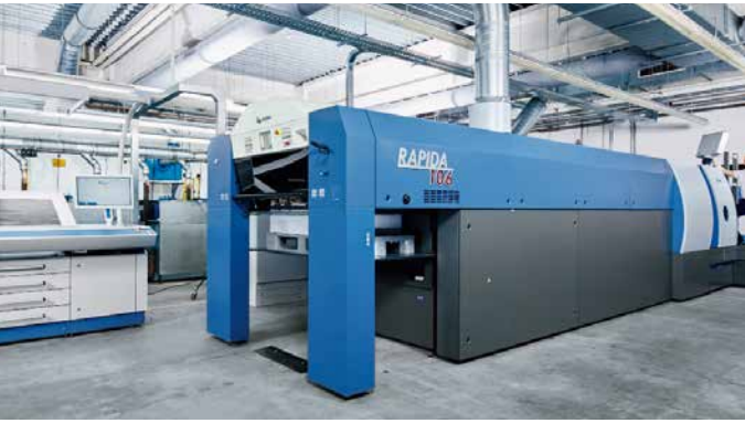
The Rapida RSP 106 enables industrial screen printing for finishing without run length limitations
