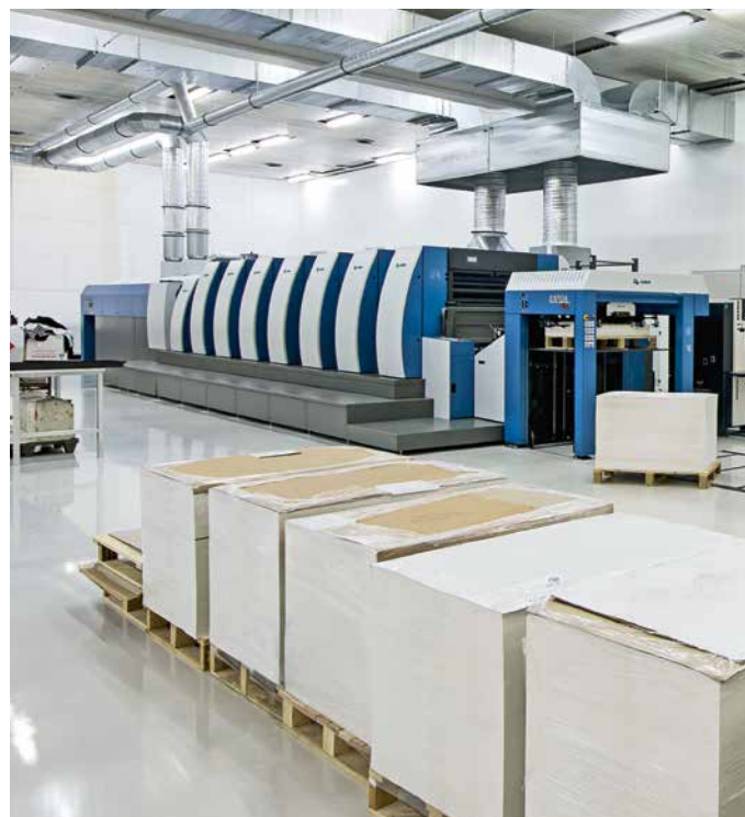
The seven-colour Rapida 106 can process either reel-fed substrates or piles
