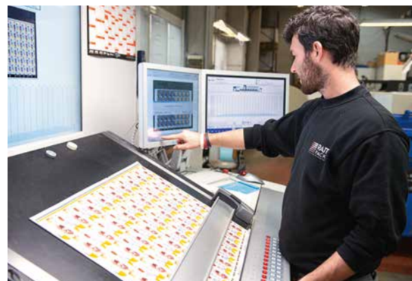
Above left: The Rapida 75 PRO features an ErgoTronic console with TouchTronic control and integrated wallscreen
