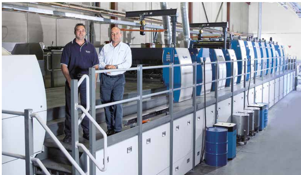
KBA Rapida 142 with 13 printing and finishing units at Anzpac in Sydney/Australia
