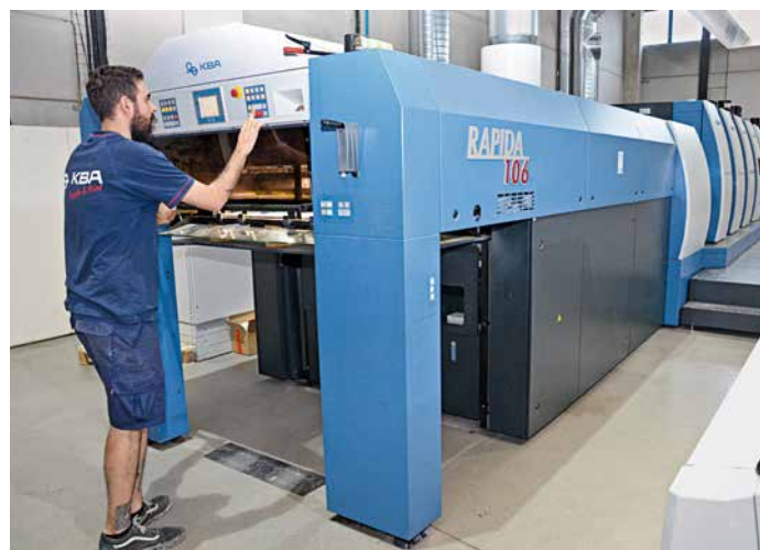
The eight-colour Rapida 106 handles a broad spectrum of commercial and packaging jobs
