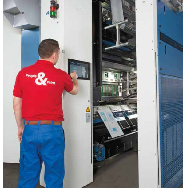
The fully automatic plate changers on the Commander CL press in Münster enable job changes for the many local editions to be accomplished in just five minutes
