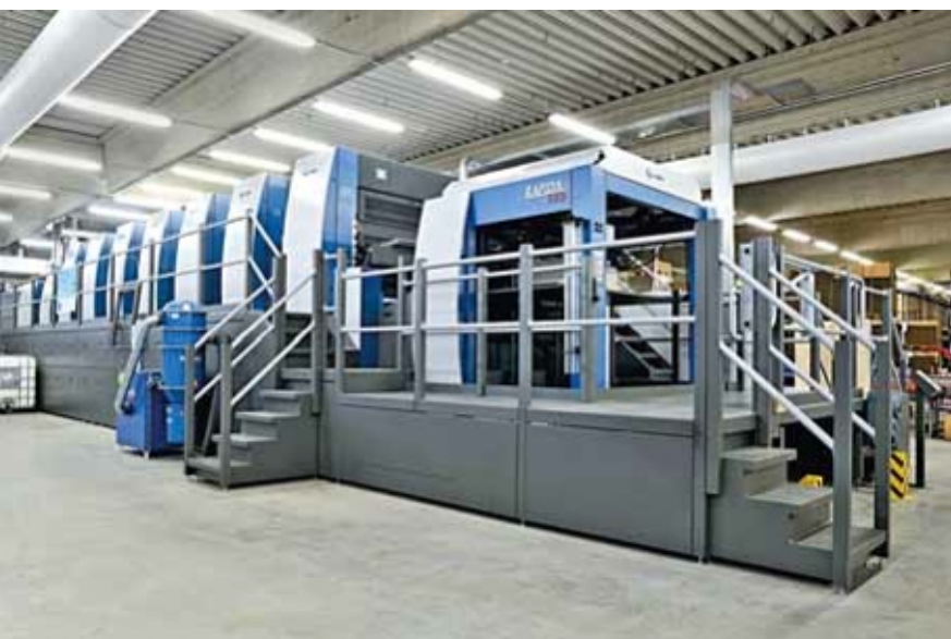
The press is raised by 630mm (24.8in) and is tailored exactly to the company's packaging production needs
