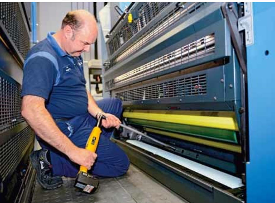
A simple battery-powered screwdriver makes changing blankets a lot easier
