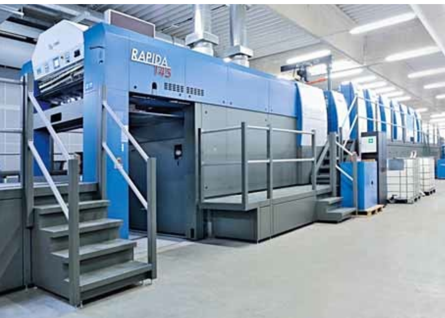
The seven-colour Rapida 145 with coater is the productive heart of Pokart's cutting-edge production hall
