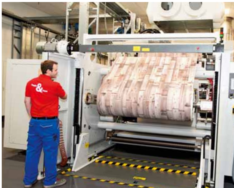
Above: Automatic webbing-up is one of the strengths of the KBA RotaJET for industrial printing
