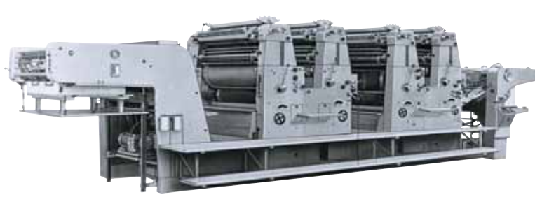
Below right: The five-cylinder system dominated in the past with all of its cons. Shown here a PVO 6 from 1957
