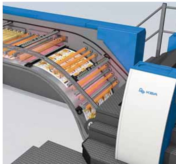
When it comes to energy efficiency there have been major advances in drying. Shown here a diagram of a VariDry BLUE drying system in the delivery extension of a Rapida 106
