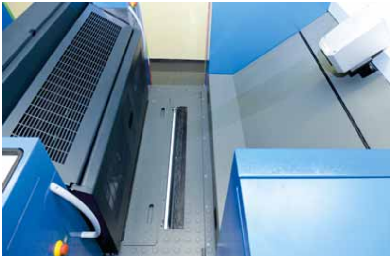
KBA offers a raft of automation modules, also for quality assurance (inspection, colour control, PDF editing). Shown here the QualiTronic camera for inline colour control
