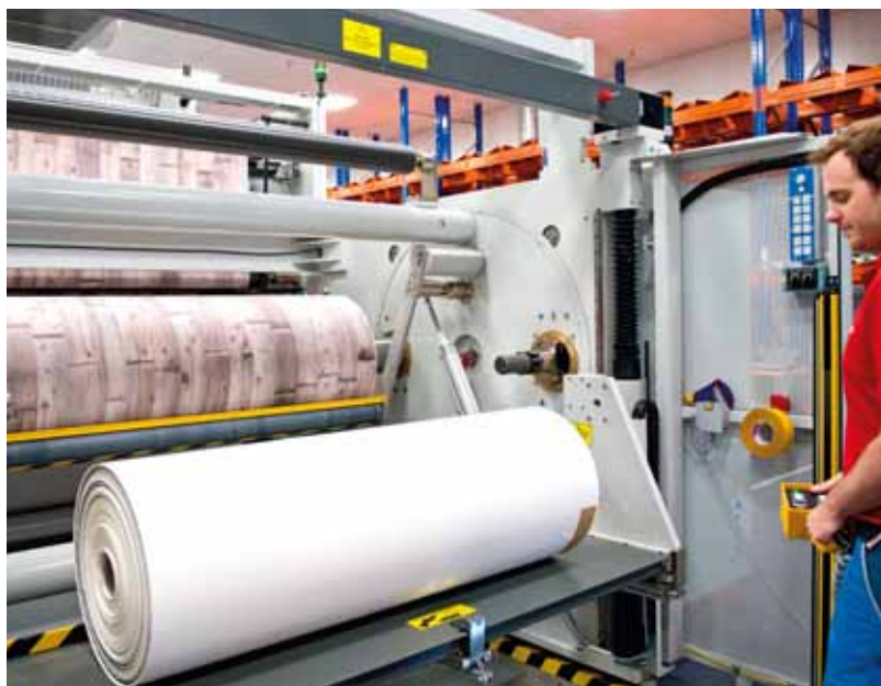
The printed reels at the rewinder are stored away during ongoing production
