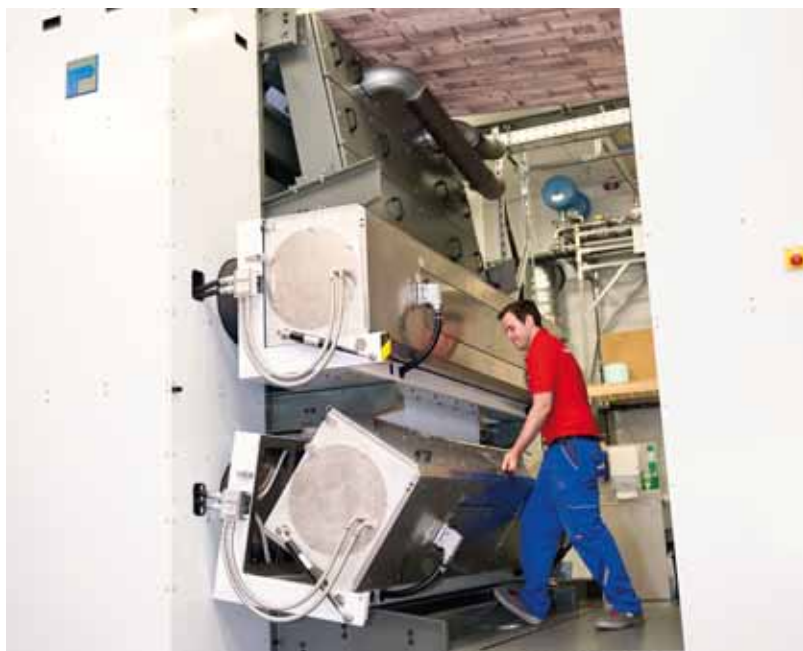
Two pivoting hybrid dryers (IR/TA) after printing
