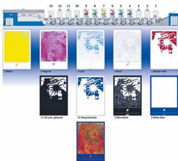
Illust. 3: Suitable for Metallure coating with hybrid finishing: Rapida 105 LTT+6+LTTL with double delivery extension and diagram of ink and coating separation using the KBA calendar from 2007 by way of example
