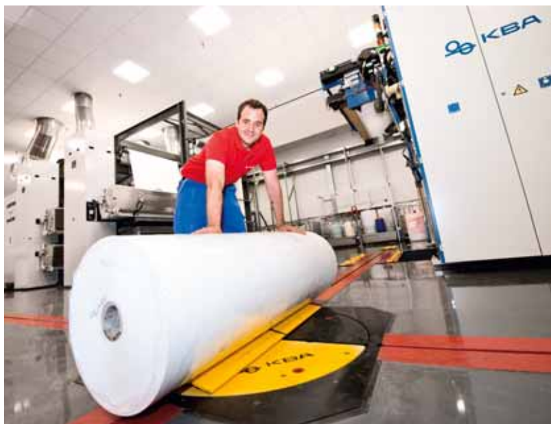
KBA Patras M supplies the KBA reelstand with 1.68m-wide paper reels
