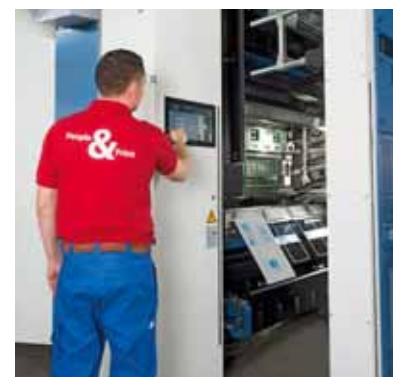
Automatic plate changing in under three minutes on the Commander CL
