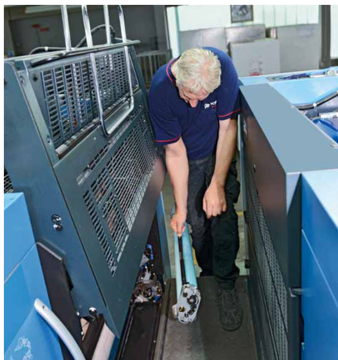
Washcloth usage is displayed on the console which allows Hubert Bauer and his colleagues to plan exactly when to change cloths
