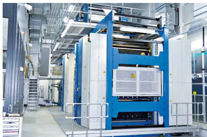
The Commander CT has four four-high towers in 6/2 configuration for up to 96 pages in tabloid format and a centrally positioned jaw folder
