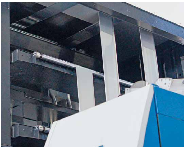
Web splitting – here with three ribbons aligned to the individual images – is one of the material-saving options for the KBA ColdFoil Infigo SF110 system
