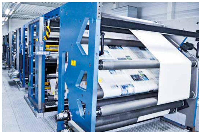
The web press' superstructure is equipped with numerous turner bars and splicing heads for maximum product flexibility
