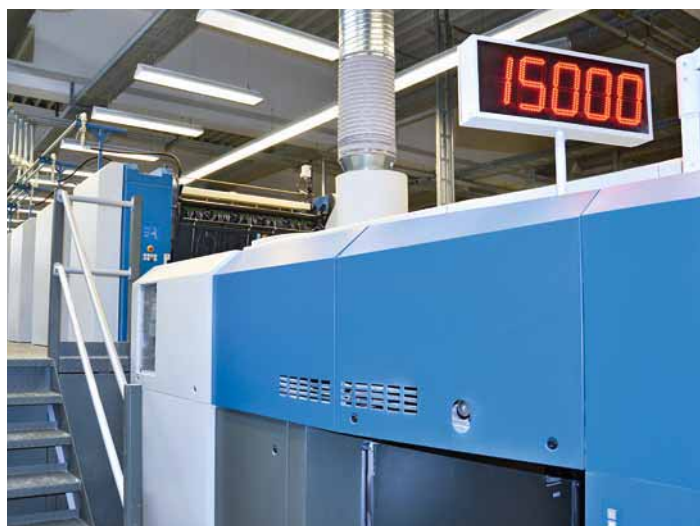
With speeds up to 15,000sph in 4-over-4 perfecting, the long large-format Rapida matches the performance of modern medium-format presses
