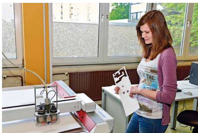
Packaging presentation samples can be produced before the main job using a cutting plotter
