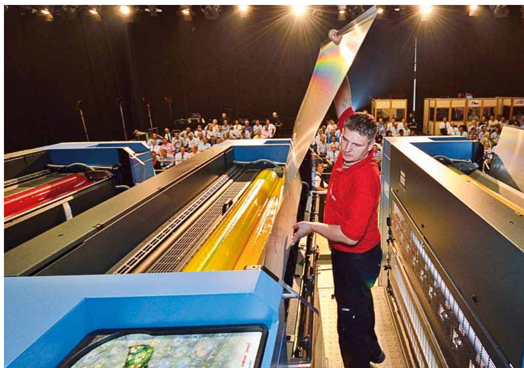
During press demonstrations Hendrik Gasch could barely keep up with mounting the plate-loading cartridges with plates for the next job, given the frequent and fast job change ensured by DriveTronic SPC
