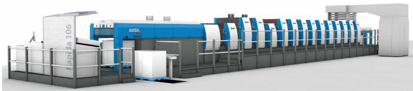
The Rapida 106 with ten inking units, double-coating technology and cold foil finishing will soon deliver outstanding effects in packaging printing at Yuri Gagarin printing house in Bulgaria
