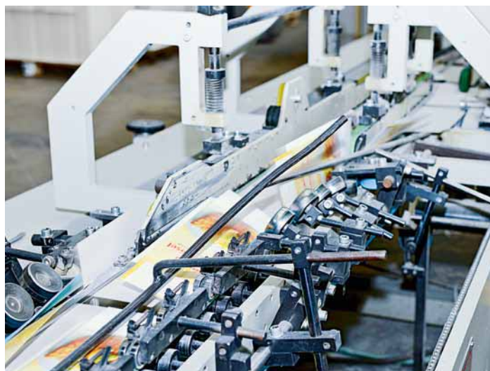
Three modern folding gluers ensure that the products are processed fast. They are equipped with various additional extras to add the finishing touches the end products
