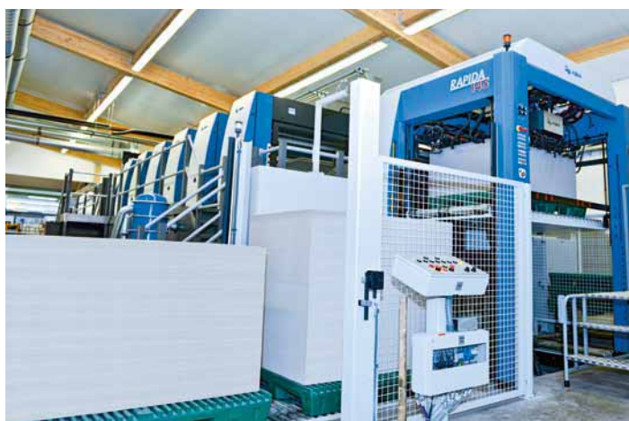
The plinth-mounted Rapida is integrated in an automated logistics system
