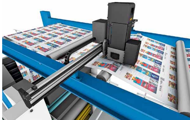
Inkjet retrofit: Crossbeam for the Kodak Prosper S30 inkjet imprinting system and cameras in the superstructure of a KBA offset press. The photo shows the standard variant with one print head. Two or more print heads are also possible to cater for a larger imprint area or higher production speeds
