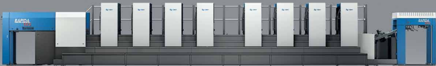
The new Rapida 105 is also available as a perfecting press for 4-over-4 or 5-over-5 printing
