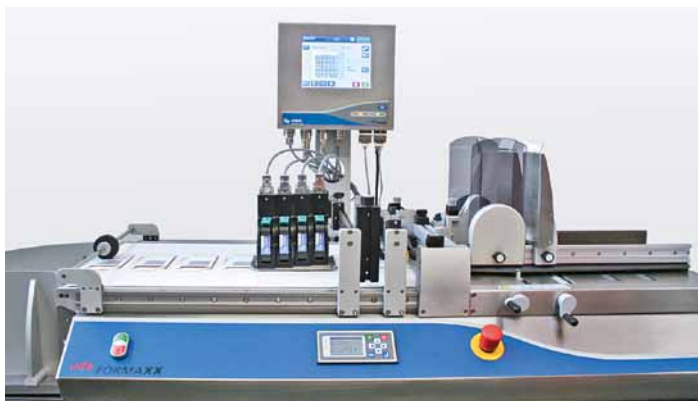
Embedded in the udaFORMAXX feeder system, the betaJET verso is ideally suited to marking folding boxes, blanks and outer boxes
