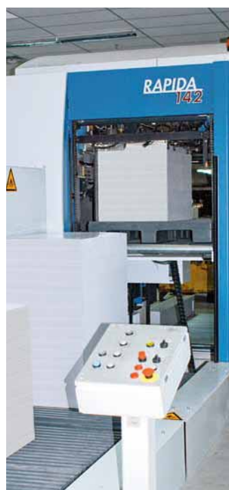
A special feature of TWP's Rapida 142 is the automatic pile change at the feeder
