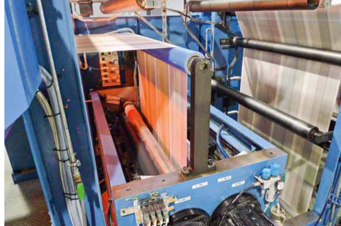
A view from above: the double-coater for coating both sides of the web is positioned directly above the Cortina printing tower
