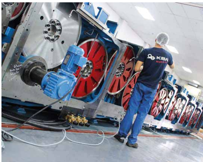
After the substructure boxes are assembled, the printing units can be mounted
