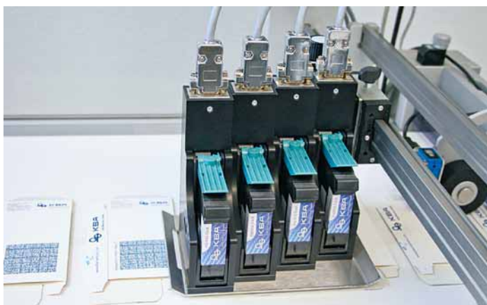
Up to four freely cascadeable printing heads can handle printing widths up to 2in (50.8mm)
