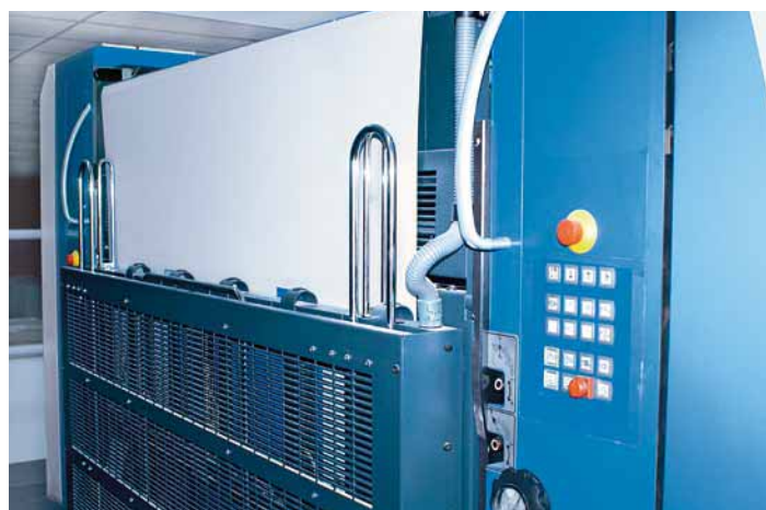
Automatic plate changing ensures fast job changes
