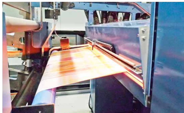
Coating with the approx. 1m (3.28ft) long IR/hot-air dryer from Eltosch is possible with nearly all types of improved stock
