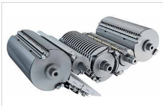
The Rapida 105 features the same cutting-edge three drum sheet perfecting system found in the high-end Rapida 106
