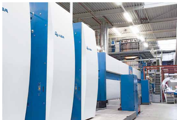
The KBA C56 SG with a maximum web width of 2,280mm (89.76in) is the only 56-page short-grain web press on the market
