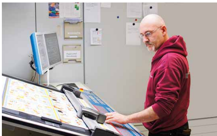
At the console printer Andreas Bayer carries out a colorimetric calibration of the colour control imaging photometer/colorimeter with an external measurement of the colour control strip
