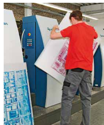
Marcus Laubach loads the plates for the next job into the changer while production is still running
