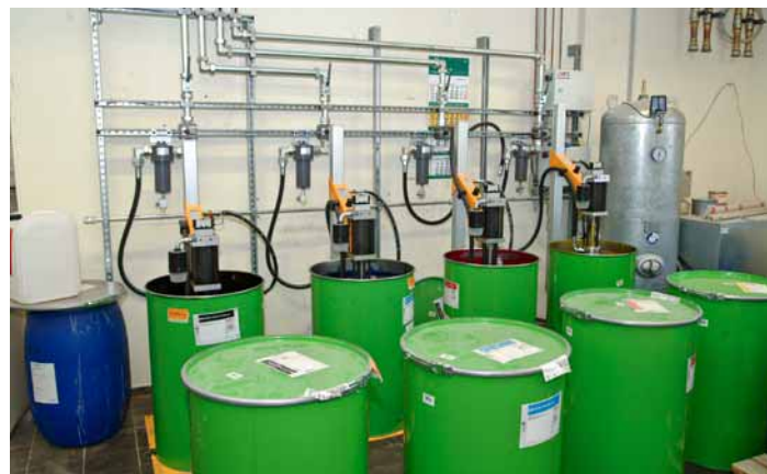
How it should be: the eight-colour press is equipped with an automatic ink supply, which always ensures fresh ink and lets the printers concentrate on printing
