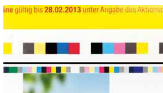
Measuring patches set for Instrument Flight in the Rapida (above, now also 3 x 3mm), System Brunner colour control strips for QuadTech CCS in heatset (below)
