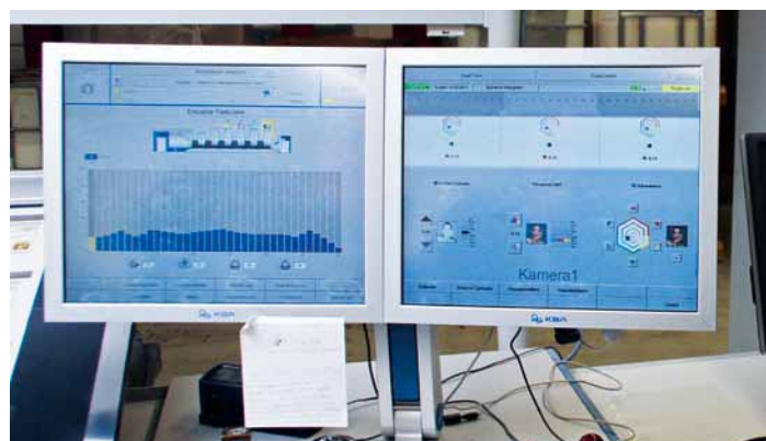
Both touchscreen monitors are active. Right is the Instrument Flight Balance Navigator with its hexagonal colour space diagrams and left the position of the colour rule including a reminder to wash the blankets
