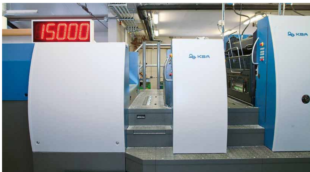
Lönneker works with a standard output of 15,000 sheets/h. Although the press can be run at higher speeds, this does not make sense when printing short runs
