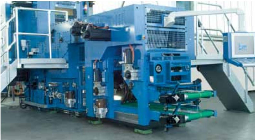
A pneumatic belt-tensioning system in the folders ensures consistent belt tension and substantially reduces belt abrasion
