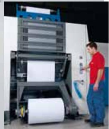
The unwiner developed by KBA for the RotaJET has an integrated controlled infeed unit for exceptionally precise web tension, and alongside automated webbing-up boasts other features hitherto rare in digital presses
