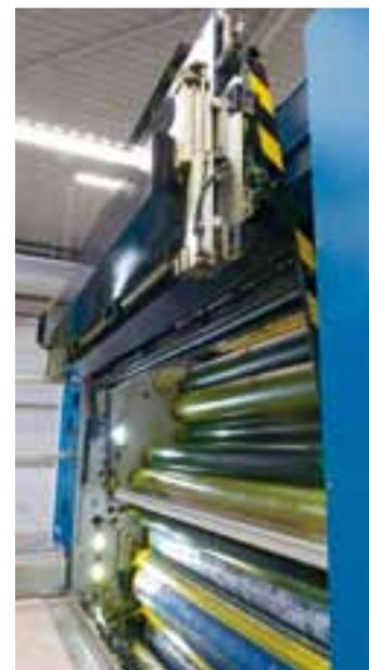
All new C series double-circumference presses are offered with an optional automatic plate-changing system that can change all the plates in an entire press line in just two minutes
