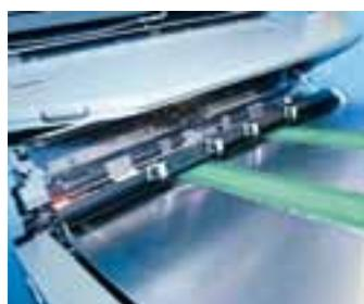
The feeder board for the Rapida 145 has just two suction belts and the proven DriveTronic SIS sidelay-free infeed adopted from the Rapida 106
