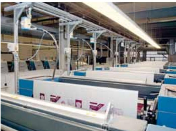
The eight-colour Rapida 106 is connected to an automatic ink-pumping system, but the six-colour (in the background) is not because it is often used for special colours
