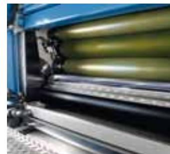
With KBA RollerTronic automatic roller locks, all the inking rollers can be set and adjusted automatically in less than two minutes by push-button at the console
