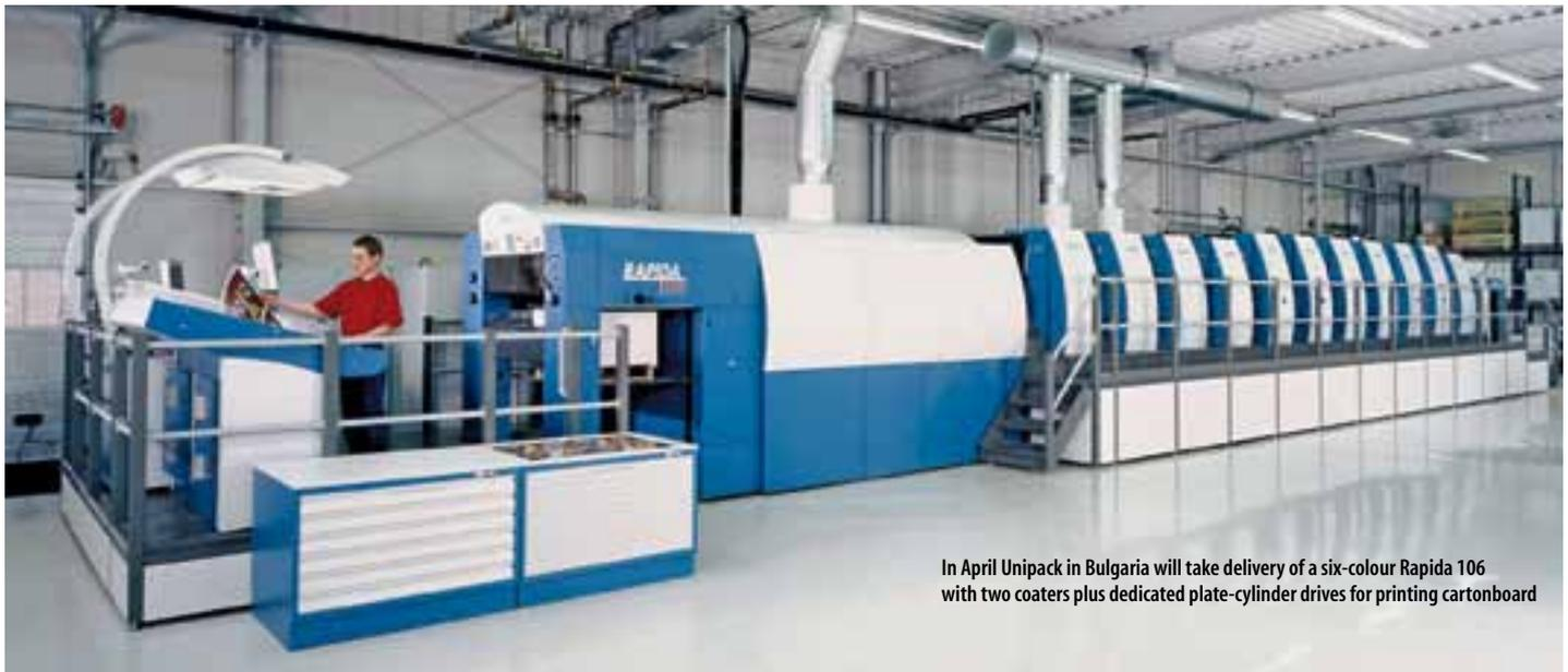
In April Unipack in Bulgaria will take delivery of a six-colour Rapida 106 with two coaters plus dedicated plate-cylinder drives for printing cartonboard
