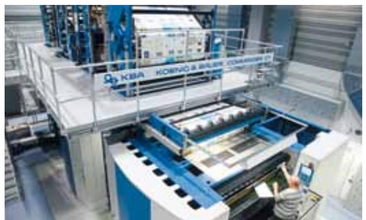
Ultra-fast edition changes thanks to convenient lifts that provide optimum access to printing couples and PlateTronic automated on-the-fly plate changers
