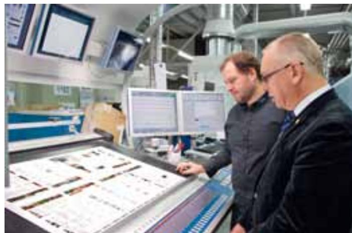
For System Brunner's Daniel Würgler (r), pictured here with Jordi plant manager Stefan Müller at the console for the Rapida 106, the installation in Belp was a milestone, since Jordi was the first to install KBA QualiTronic colour control in tandem with Instrument Flight
