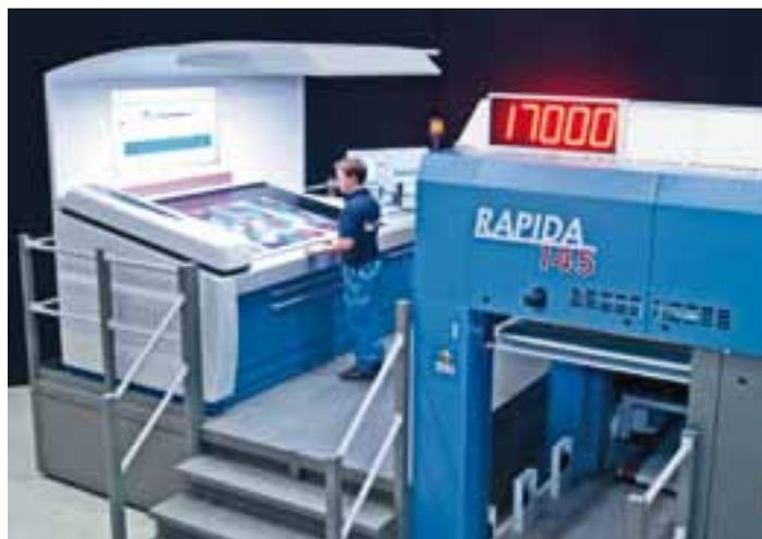
View across the new Rapida 145's overhead venturi delivery to the new ErgoTronic console with integrated measurement and control systems
