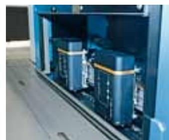
Digital meets offset: the Rapida 105 is equipped with inkjet heads from Atlantic Zeiser for personalised imprints and product coding
