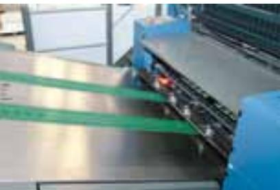
The elimination of rollers and brushes at the feeder board is a neat solution; the red light is emitted by the DriveTronic SIS sidelay-free infeed system
