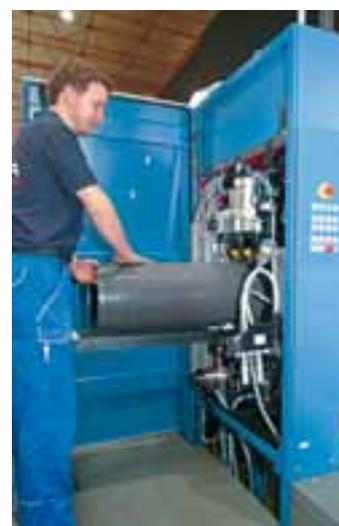
The Rapida 145's new coater supports simultaneous forme changes via DriveTronic SFC, and sleeves on the anilox rollers can be replaced single-handedly in no time
