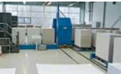
The automated pile-logistics system for the three large-format Rapidas includes a shuttle trolley that conveys the prepared piles to buffer stations at the feeders
