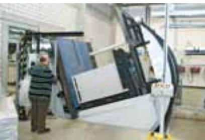
All the piles are transferred to nonstop pallets by a pile turner at the diverter between the materials store and the press room
