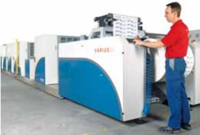
KBA-Metronic's udaFORMAXX separating system for folding cartons has an integrated, freely programmable betaJET thermal inkjet unit for addressing, offline coding etc
