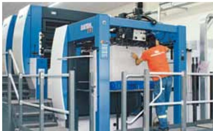
The large-format Rapida which came on stream in March 2011 is mounted on a plinth to accommodate the higher piles common in board printing
